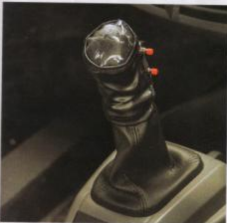
The red buttons on this gear lever operate the clutch.
